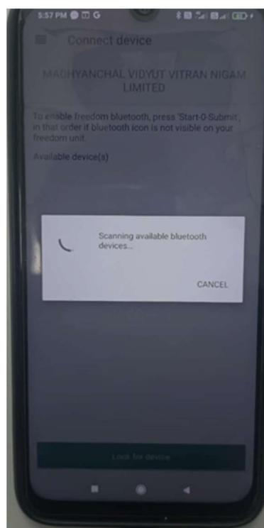
Mobile have to in Bluetooth range of provided by discom “**In-Home Display Unit**” (**freedom unit**) and Sahaj Liberty app will automatically connect to the **In-Home Display Unit**” (**freedom unit**), app will be read ABC code automatically from meter and process the ABC code.
